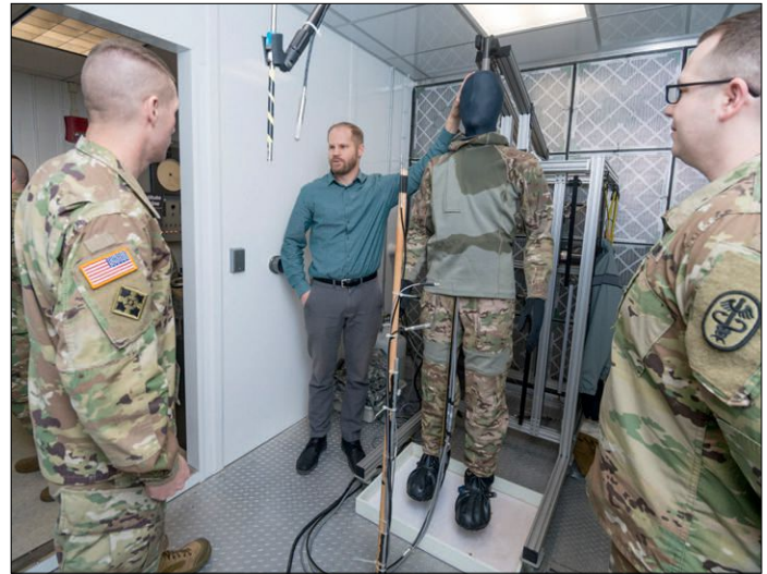
The U.S. Army Research Institute of Environmental Medicine researcher, Timothy Rioux, demonstrates the principle of evaporative resistance in textiles using the Newton manikin. Rioux explains how the specific type of clothing worn by a warfighter affects the heat exchange between the human body and the environment they are in. (USARIEM)
