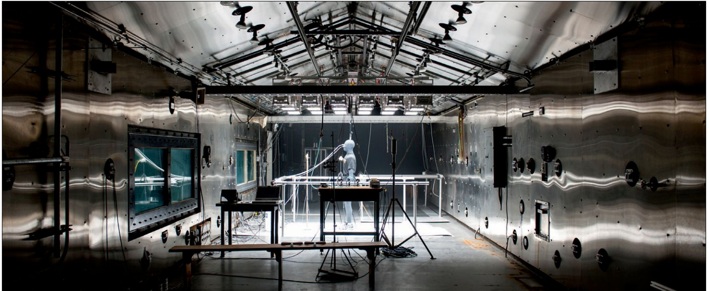
The Newton thermal manikin was positioned inside the environmental chamber where the solar tests were conducted. Throughout the experiment, 30 independent zones on the manikin were measured to demonstrate the extent and distribution of heat gain, providing a detailed understanding of how each body part was affected. (USARIEM)
