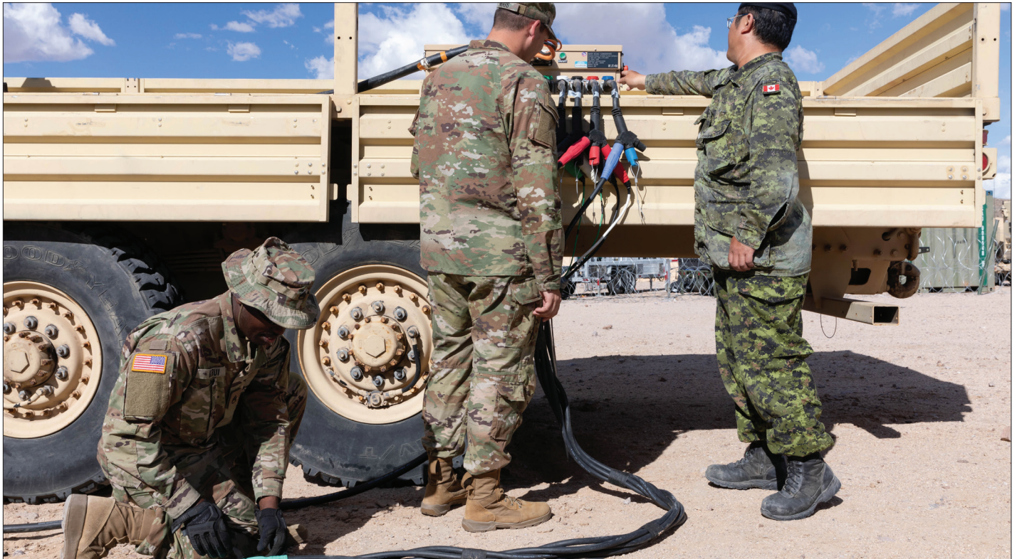
A 15-person component of the Army's 11th Air Defense Artillery Brigade carried out an operational assessment of Secure Tactical Advanced Mobile Power (STAMP) last August at Fort Bliss, Texas. STAMP technology allows multiple vehicles to network their electrical systems together as a microgrid. Lightweight and fast-forming, STAMP aims to rapidly increase U.S. forces' fight and sustainment capability when engaged forward (U.S. Army photo).
