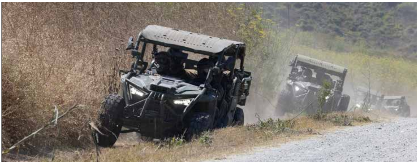
U.S. Marines drive the Ultra Light Tactical Vehicle (ULTV) during an operational new equipment training at Marine Corps Base Camp Pendleton, CA in July 2023. The ULTV is a modular, off-road utility vehicle which can be configured to provide logistical support to the Fleet Marine Force, perform casualty evacuation, command and control, and electronic warfare missions. Marine Corps Systems Command's Program Manager for Light Tactical Vehicles started fielding the ULTV to Marines in June 2023. (U.S. Marine Corps photo by Sgt. Nicolas Atehortua)
