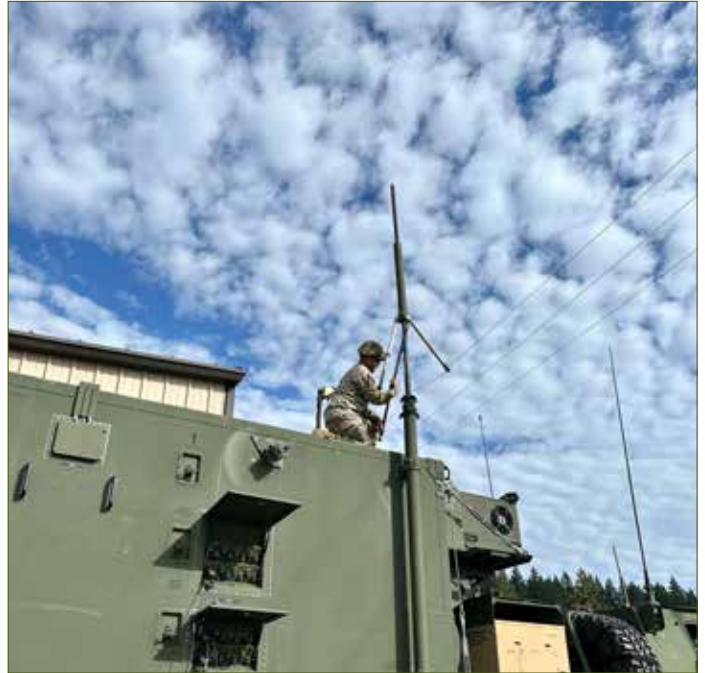
A Soldier with 1st Stryker Brigade Combat Team, 2nd Infantry Division (1-2 SBCT) attaches an antenna to one of the Mobile Command Platforms (MCP) during the Command Post Integrated Infrastructure (CPI2) Limited User Test at Joint Base Lewis McChord, Washington. The MCP is one of the command post function support vehicle platforms to enable command and control on the move. (PEO C3T)
