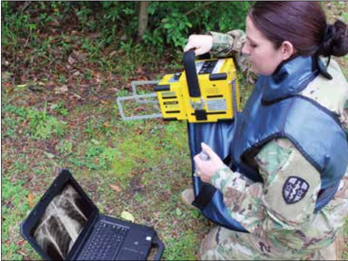
X-Ranger Wireless is a battery-powered portable digital radiography system specially designed for military use.
