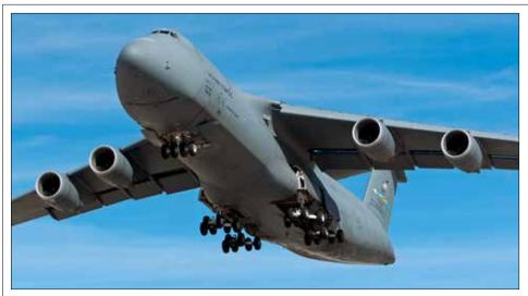
GE re-engined the C-5 with its F138 propulsion system, creating the C-5M Super Galaxy with multiple improvements, including increased range and decreased maintenance man-hours. (Photo courtesy of One Mile High Photography)
