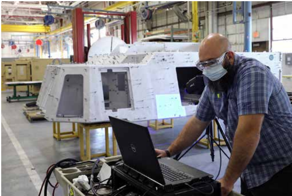
Benjamin Thomason, metrology team lead, Aviation and Missile Center (AvMC), U.S. Army Combat Capabilities Development Command (DEVCOM) operates a structured blue light scanner to evaluate the surface geometry of a turret that is being converted into an Extended Range Cannon Artillery (ERCA) turret at Letterkenny Army Depot (LEAD). The scans provide mechanical engineers at LEAD with a baseline for the turrets as received from the customer, and will be used as a comparison to the customer provided model to evaluate the work to be executed and areas of concern. The partnership between LEAD and DEVCOM focuses on implementing technologies at the depot level that they might otherwise not have access to. (U.S. Army photo by Pam Goodhart)
