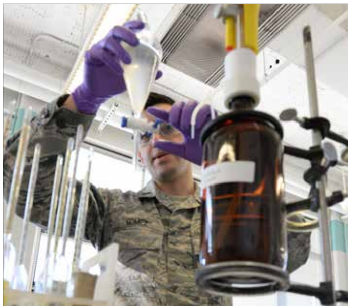
1st Lt. William Gomez, Aerospace Fuels Laboratory deputy chief, checks for separation of fuel and water in a sample at the Quality Surveillance Fuels Lab, Wright-Patterson Air Force Base, OH. The additive being tested for prevents water in the fuel from freezing as it separates in flight. (U.S. Air Force photo by Michelle Gigante)
