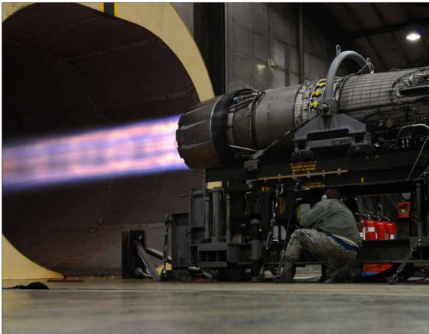
Staff Sgt. Daniel Gallentine, 20th Component Maintenance Squadron jet engine craftsman, inspects a jet engine at the engine test facility, Shaw Air Force Base, SC. While the engine was at 29,000 pounds thrust capacity, Gallentine checked for oil and air leaks as well as any vibrating parts to ensure all components were working properly. (U.S. Air Force photo by Airman 1st Class Jensen Stidham/Released)
