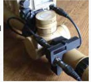
The Eagle enables the shooter to gain firing solutions in canted firing positions and interfaces with STORM, RULR, PLRF, and RAPTOR LRFs—in addition to thermal weapon systems (INOD BLK III, HISS)—to further decrease time to engagement. The Eagle has been selected for testing in the Army's Soldier Enhancement Program.
